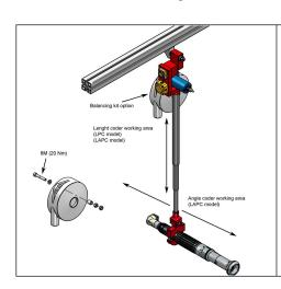
Attach the arm as shown in the image. Take care to orient the pivot for the required work area.
