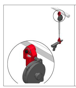
Attach the arm as shown in the image. Take care to orient the pivot for the required work area.
