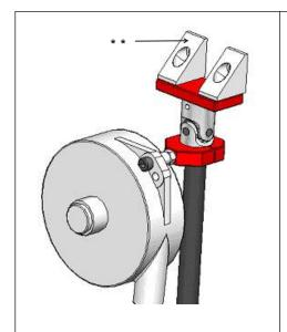
Attach the arm as shown in the image. Take care to orient the cardan for the required work area.
