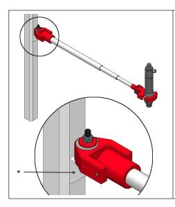
Attach the arm to a post as shown in the image. Take care to orient the pivot for the required work area.
